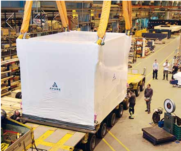
Arrived: the new graphite production center in Bonn received its core element after fifteen months of construction, the largest cold isostatic press in the world.
